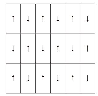
When installing this product, as indicated in the figure above, place the adjacent tile on the opposite direction.
